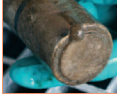
Sensor without ultrasound cleaning system After 16 Days
