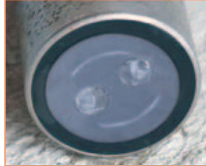
Sensor with ultrasound cleaning system After 16 Days
